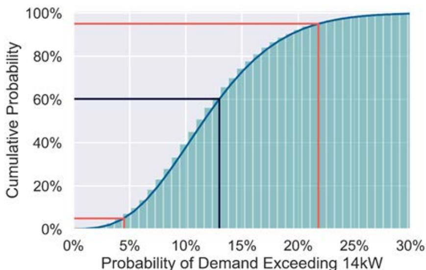
Figure 6: Probability of demand from 15 electric vehicles exceeding 14 kW
